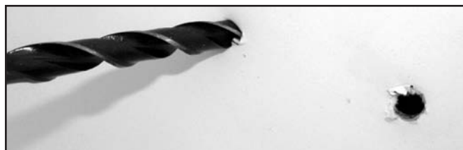
8. Now (heart pounding) drill the holes. We suggest not center punching, but, instead, starting with a small (1/8" or so) super-sharp bit. Once the holes have been drilled, it's a good idea to brush-apply a little primer to the exposed bare metal surfaces.
