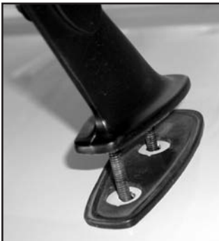
10. Position the gaskets, then place the spoiler, with stanchions and studs installed, through the holes. Install the Palnuts finger-loose, then move the gaskets into exact position (raised lip showing all around). Then snug the Palnuts.
