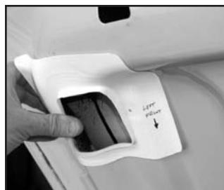
14. Ok, Vern, you have a '74 decklid on your '70 225 CID 'Cuda that you've made into a '71 HemiCuda ragtop. And the '71-only factory-stamped spoiler bracket cutouts aren't there—or are wrong. Where to make the cutouts? First Place has these incredible 3-dimensional templates to solve that problem. With care, a nibbler, or small (3") cutoff wheel. You can do a neat job without damaging the outer skin. Several other versions are available, too.
