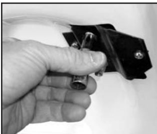
11. Thread in the adjusters, and attach the reinforcement plates (two SEMS screws to the U-nuts in photo 9). Now back out the adjusters, as shown, until they are just flush with the brackets. Then install the washers and nuts.
