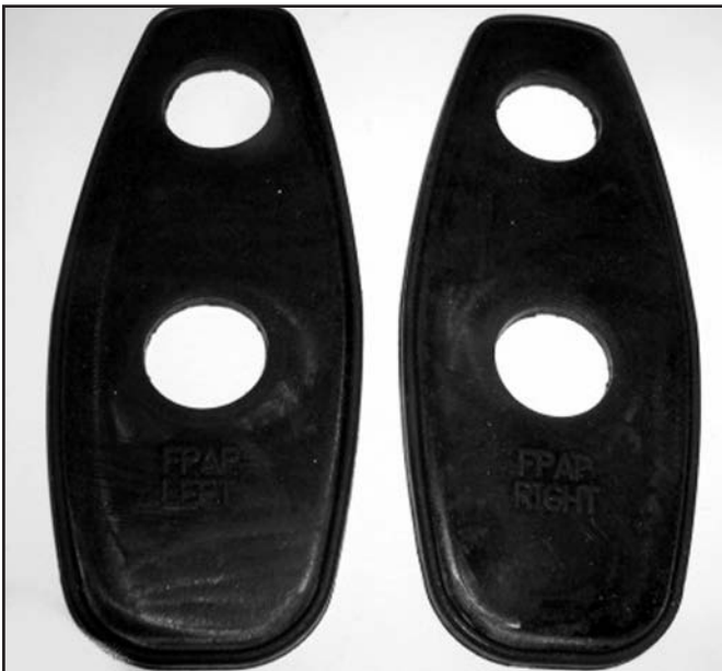
5. Gaskets are correct "handed" (i.e., different left and right, and have correct raised lip.
