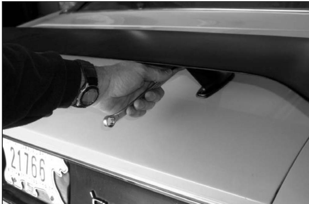
**12. Adjust the angle of attack as you wish (steeper angle for 175 MPH+) and you're done!**
