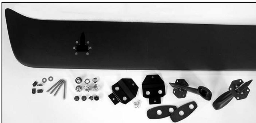
**2. First Place Auto Products to the rescue! The UPS man brought us their 100% complete Go-Wing kit. Most importantly, all dimensions are same as original, i.e., thickness, taper, length, width, height, crown, and curve. The spoiler blade itself is molded in black ABS plastic (as original).**
